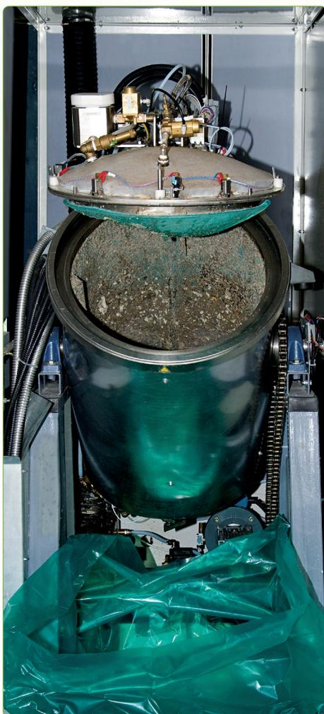
Celitron's compact medical hazardous waste solution, the Integrated Sterilizer & Shredder, is a large steam sterilizer with an integrated shredder, designed for on-site conversion of biohazard waste in hospitals and clinics, complying the EU and WHO recommendations.
