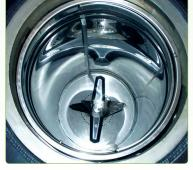
The blades are mounted on the shaft and designed to shred waste such as sharps, dialyzers, syringes, papers, cloth, plastic and glass. The 4 kW motor is sufficient to rotate the shaft with an RPM of 400-1700 for various operations.
