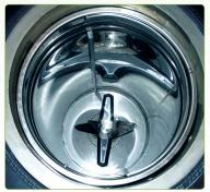
The stainless steel vessel is fitted with a motor-driven shaft and the powerful shredding / crushing blades that can rotate in two directions to reduce the size and volume of the waste down to 20%.
