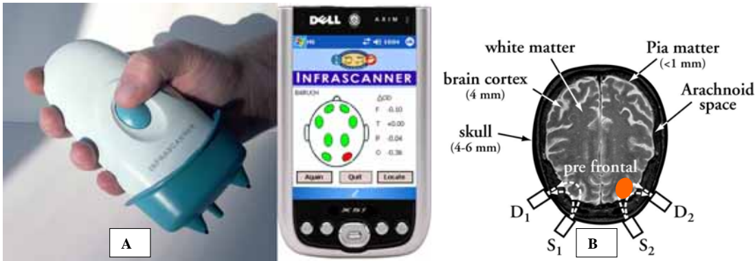
Fig. 2 The Infrascanner TM (A) is a portable tomograph. The technique for detecting a hematoma (B) is based on the different levels of light absorption by the left and right hemispheres of the brain. In the normal state, both hemispheres absorb light identically. When an extravascular blood clot is present, the local concentration of hemoglobin rises and the optical absorption constant increases in proportion to the decrease in the reflected light component. The difference is established using sensors and detectors that are symmetrically positioned on both sides of the cranium.
