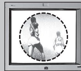
Arthroscopy/Urology (Circle Size) Arthroscopy Ø 4 mm/f = 18 mm
